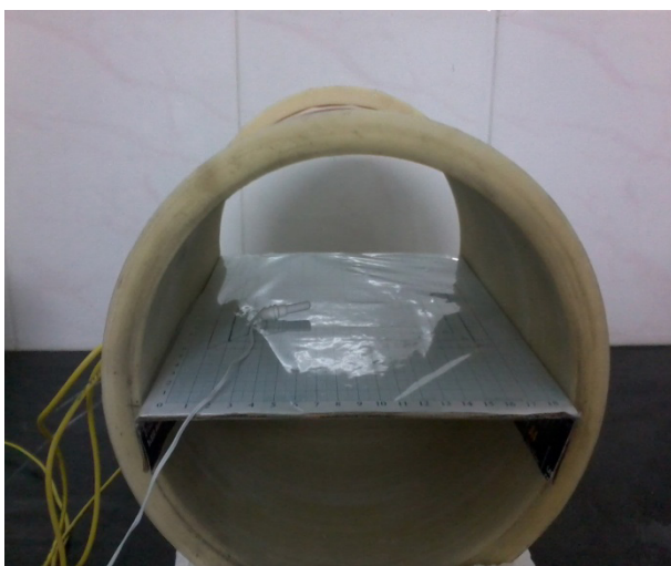
Figure 4: Homemade solenoid coils with calibrated plate. Digital thermometer probe located at the center of solenoid.
