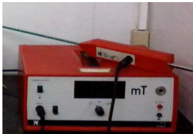
Figure 3: Teslameter and its probe
