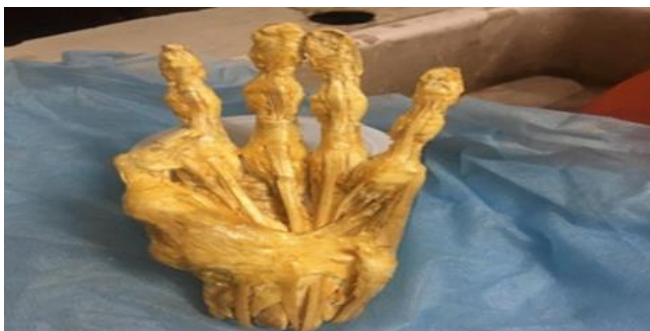
Figure 8: finishing of specimen & paint with melamine for hardening (mix of Chloroform + melamine along with hardner in equal ratio)
